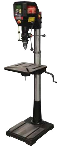
The 18 in. Nova Voyager DVR drill press has been introduced by **King Canada**. Features of the smart drill press include a direct drive 1.75 hp high torque motor with no pulleys or
